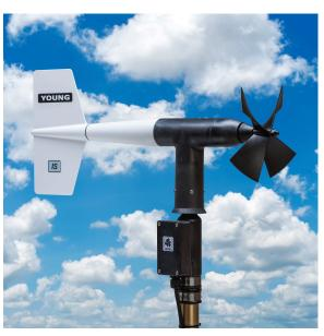
The wind direction sensor is a durable molded vane. Vane angle is sensed by a precision, long-life potentiometer housed in a sealed chamber.
